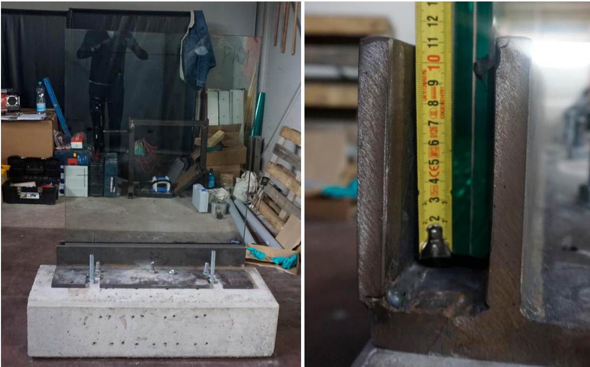
Image 4 Test setup (left) and fixing height of the glass (right)
